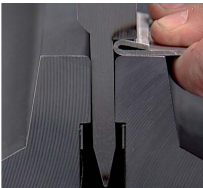
Pre-bend and flattening in the same tool.
